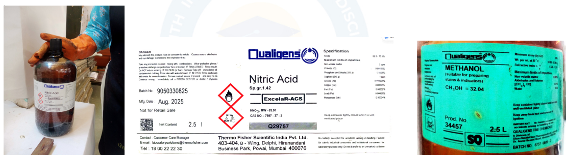
Nitric acid is used on Zinc plate & Litho stone etching.
