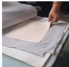
Damping printing paper in blotting paper.
