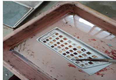
Etching process on zinc plate
